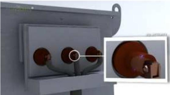
PD can occur at any point in an insulated system.
