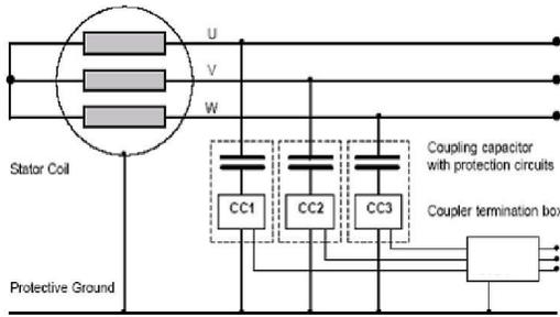
Picture: capacitive couplers and termination box as fixed equipment on the motor for scheduled on-line measurements
