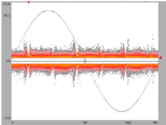
Picture: PD signal is embedded into noise and measurement settings are not well tuned in
