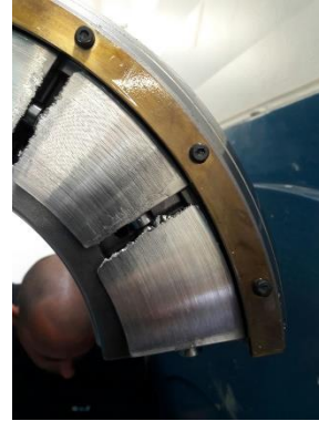
Fig. 17 – Rubbing of bearing thrust pads
