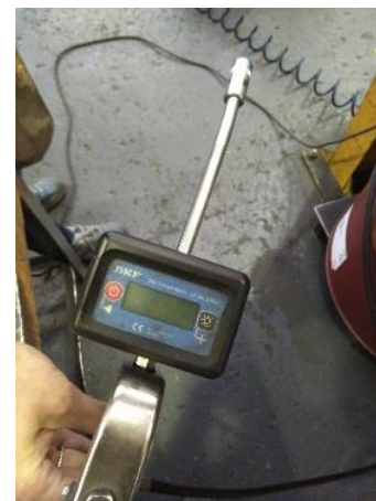
Fig. 9 – Example of grease flow meter
