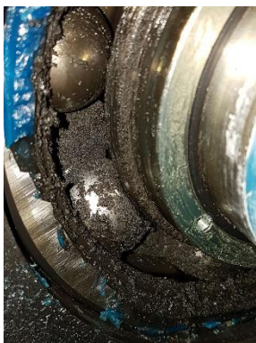
Fig. 16 – Burnt grease due to stray currents in bearing
