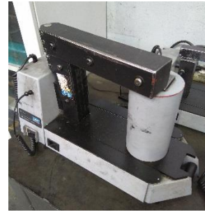
Fig. 12 – Induction heating machine for bearings
