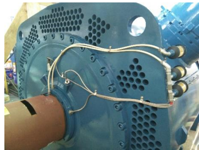
Fig. 6 – Medium voltage flameproof motor fitted with automatic lubricators
